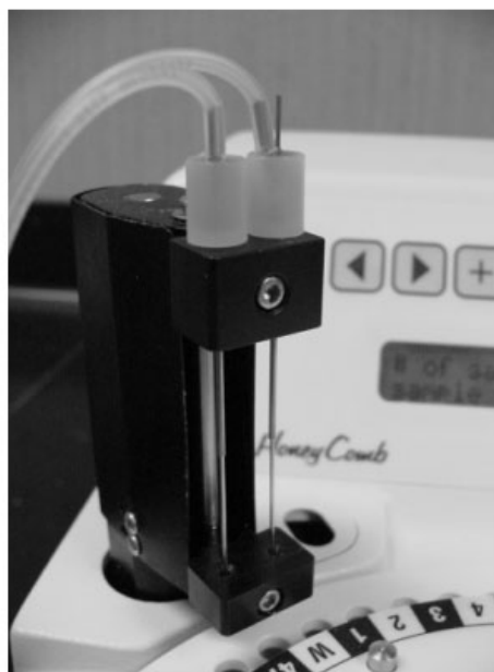
F5. Two vacuum needles installed in the HoneyComb fraction collector, each attached to the vacuum line. This arrangement collects samples from two probes in one animal, or one probe in each of two animals.
