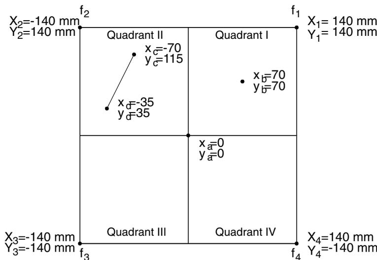
exactly equidistant between each of the four support points (namely, at  $x_a=0, y_a=0$ , the center of the coordinate system), then the forces sensed at the four support points will sum to the force in the center. If the applied force is moved along a diagonal from  $x_a=0, y_a=0$  toward  $(X_1, Y_1)$ , the  $f_1$  force at  $(X_1, Y_1)$  will rise and the  $f_3$  force at  $(X_3, Y_3)$  at the opposite end of this diagonal will fall in proportion to the distances involved.
