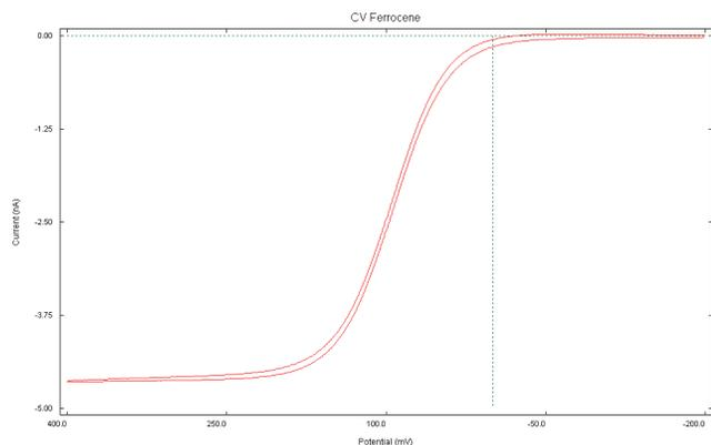
Figure 1. Cyclic voltammogram of 1 mM Ferrocene in 0.1 M TBAP/Acetonitrile with a 10  $\mu$ m platinum electrode at a scan rate of 50 mV/s. This is raw data with no post-run smoothing. This is a typical voltammogram obtained with the most common size microelectrode and concentration of analyte which, in turn, gives a current in the 1-10 nA range.
