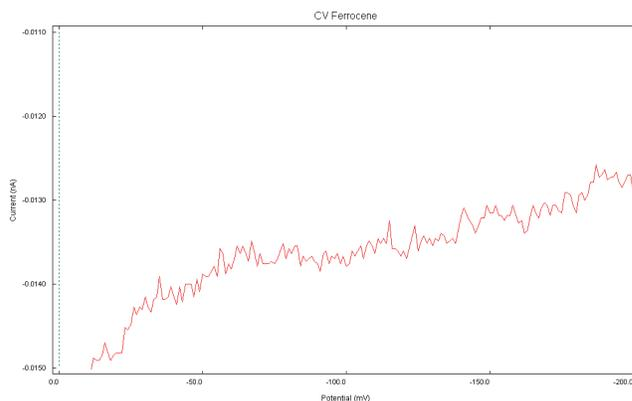
Figure 3. Expanded scale of data in Figure 2 to demonstrate noise in raw data. Note that each division of Y-axis is 1 pA.
