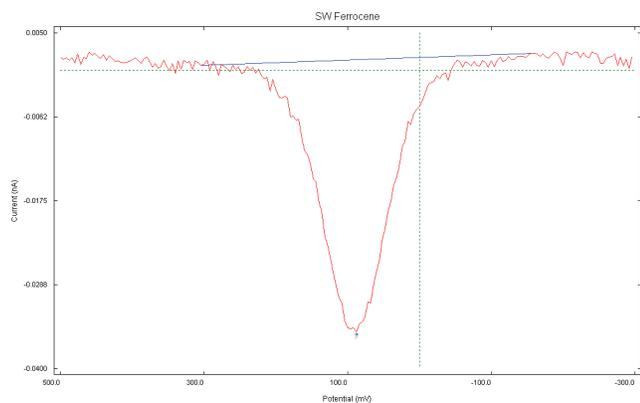
Figure 4. Squarewave voltammogram of 10  $\mu\text{M}$  Ferrocene in 0.1 M TBAP/Acetonitrile with a 10  $\mu\text{m}$  platinum electrode at a frequency of 15 Hz. This is raw data with no post run smoothing. Normally, smoothing is performed after the run to reduce noise and give a more reproducible peak measurement. The peak height is 36 pA.
