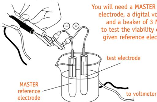
You will need a MASTER reference electrode, a digital voltmeter and a beaker of 3 M KCl to test the viability of any given reference electrode.
