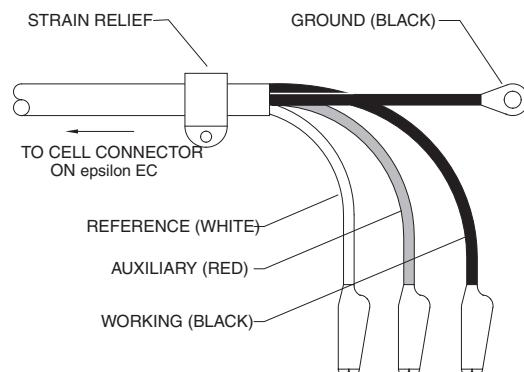
There are 3 electrode leads and 1 grounded (shielding) lead. The color code is:
