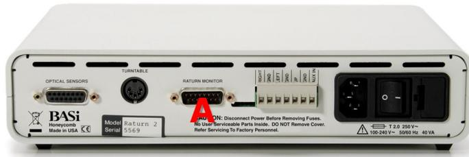
2. Connect a tan Return monitor cable from the monitor port on the back of each Return controller (**A**) to one of the monitor ports on the back of the Activity Monitor controller. **NOTE:** If you have an older Return with three or four colored ports, you will need to exchange the tan monitor cables for a cable with banana jacks (EW-7508 – three port; EW-7514- four port). Please contact BASi to make the exchange.
