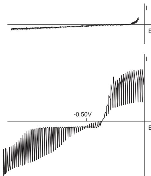
**F4.** DC polarogram of 2 mM NADP<sup>+</sup> and 2 mM NADPH in EBS.  $E_i = 0.260\text{V}$ ,  $E_f = -1.24\text{V}$ , scan rate = 5 mV/s,  $t = 1\text{ s}$ .
